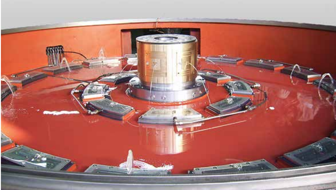
Set of bearings for rotary table Ø 4.000 mm
